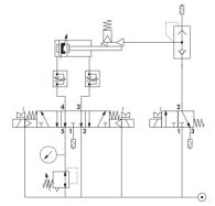
In this regard, Metal Work offers both ISO 15552 cylinders with end-of-stroke stop, which allow the rod to be retained at both ends of the movement, and the rod locks of the Secure Lock and RL Series, which allow locking even in intermediate positions.
