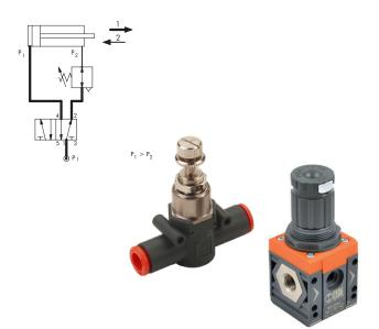
In the same way it is also possible to use the pressure regulators of the Syntesi Series that, being natively made in the quick discharge version, can be inserted between valve and cylinder, thus performing the same function as the Line On Line reducers in case superior flow rates are required.
